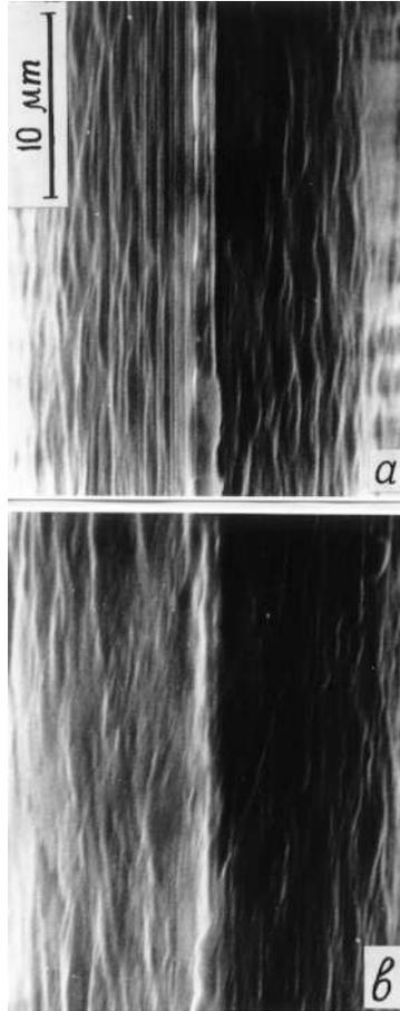
Figure 1: Micrographs of the cutting edge of the "Gillette" blade; top view of the edge [3000×]: *a* - reference specimen; *b* - test specimen.
